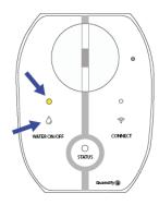
The deactivation of the alarm can be done in the app or manually by holding down the water ON/OFF button for 5 seconds. The LED will turn yellow when deactivated. Press again once to re-activate leak detection.
