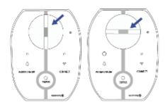
The picture on the left shows an open valve, a closed valve is shown on the right.
